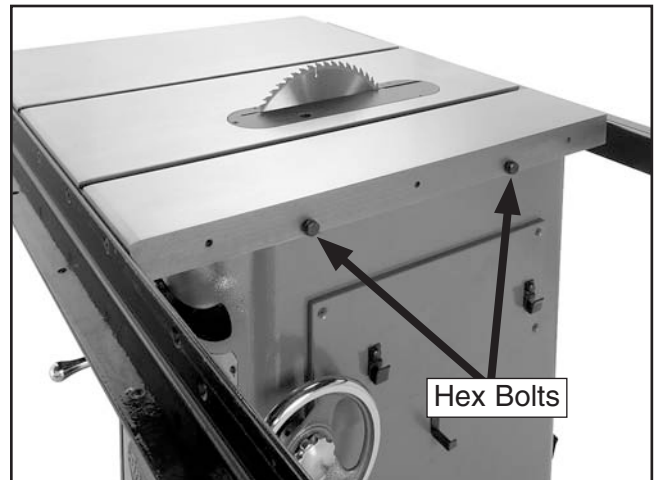
Figure 12. Hex bolts installed.
